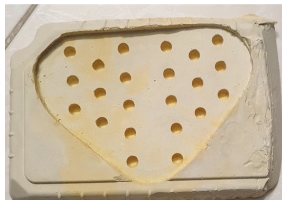
Figure 2. Mold made to produce silicone pads
