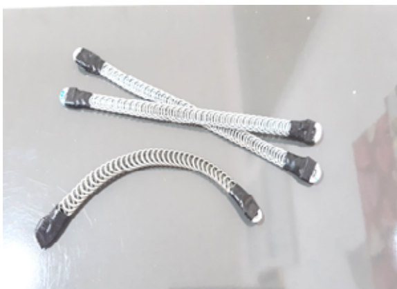
Figure 4. Springs installed in the knee and wrist area
